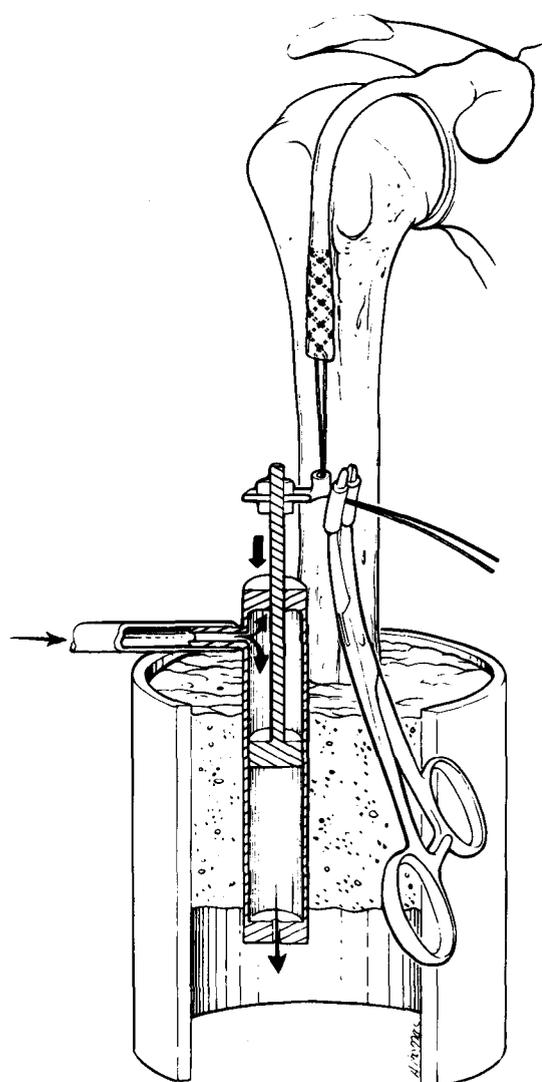
**Figure 1** Application of force to tendon of long head of biceps brachii. Air cylinder was potted adjacent to humeral shaft. Air cylinder was connected to tendon with sutures and couplers that were attached to piston of air cylinder. Activation of air cylinder applied constant force to tendon.
